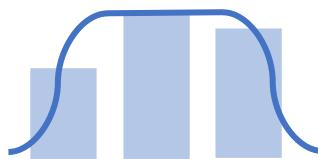
For the sake of our discussion, we will refer to the full set of bars as shown above as the "pulse", corresponding to the solid line in the diagram. The individual smaller bursts of electricity that make up the "pulse" will be referred to as "bars."
