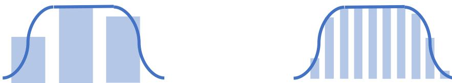
So, there will be a trade-off between the two. Most flyers will simply accept the default PWM frequency, as long as the motor runs smoothly. In tests that I have seen, there's only a 2% increase in power between the minimum and maximum frequencies. So, generally we stick to the low end of the range, as long as the motor runs smoothly, for the sake of the ESC. If it's noisy, increase the frequency to see if that stops the noise.
